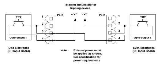
(Switch SW5 is set to W for low level alarms and set to S for high level alarms)
